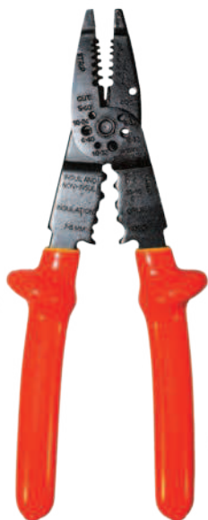
WS19 Strips and Cuts 10-22 AWG Solid or Stranded
